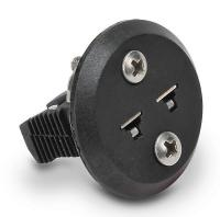
ProSense Type J thermocouple connector, miniature flat pin panel jack, 400 deg F (200 deg C), glass filled thermoplastic body, black, thermocouple material pins, 32 AWG to 14 AWG wire size range.
