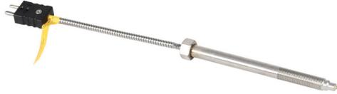
ProSense temperature sensor, Type J thermocouple, melt bolt probe, grounded junction, 6in bolt length, 1/8in tip, stainless steel sheath, 1/2-20 UNF process connection, 6in lead wire extension with 2-pin standard size plug.
