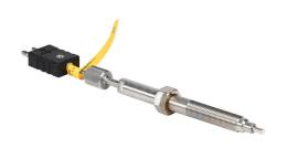
ProSense temperature sensor, Type J thermocouple, melt bolt probe, exposed junction, 3in bolt length, 0 to 1in adjustable tip, stainless steel sheath, 1/2-20 UNF process connection, 2-pin standard size plug.
