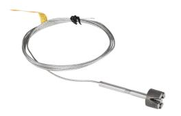
ProSense temperature sensor, Type J thermocouple, magnet mount sensor, exposed junction, 10 lb pull magnet process connection, 6ft 20 AWG wire leads.
