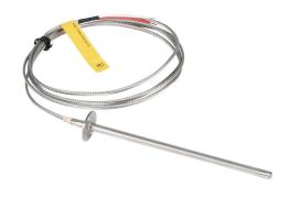
ProSense temperature sensor, Type J thermocouple, flange mount probe, ungrounded junction, 6in insertion length, 1/4in probe diameter, stainless steel sheath, mounting flange process connection, 6ft 20 AWG wire leads.
