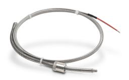
ProSense temperature sensor, Type J thermocouple, spring adjustable immersion probe, ungrounded, 1/4in insertion length, 3/16in probe diameter, stainless steel sheath, bayonet cap process connection, 10ft 20 AWG wire leads.
