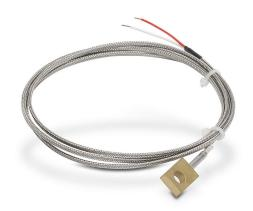
ProSense temperature sensor, Type J thermocouple, bolt-on ring, ungrounded junction, brass sheath, #12, 1/4 - 5/16in (5-8mm) screw or bolt size process connection, 6ft 20 AWG wire leads.
