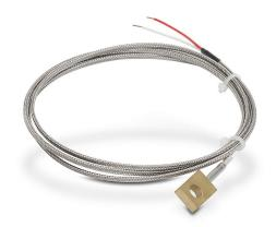
ProSense temperature sensor, Type J thermocouple, bolt-on ring, ungrounded, brass sheath, #12, 1/4 to 5/16in (5mm to 8mm) screw or bolt size process connection, 6ft 20 AWG wire leads.
