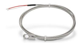
ProSense temperature sensor, Type J thermocouple, bolt-on ring, grounded junction, stainless steel sheath, #12, 1/4 - 5/16in (5-8mm) screw or bolt size process connection, 6ft 20 AWG wire leads.
