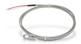
ProSense temperature sensor, Type J thermocouple, bolt-on ring, grounded, stainless steel sheath, #12, 1/4 to 5/16in (5mm to 8mm) screw or bolt size process connection, 6ft 20 AWG wire leads.
