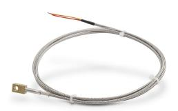
ProSense temperature sensor, Type J thermocouple, bolt-on ring, ungrounded, brass sheath, #6 to #10 (4mm to 5mm) screw or bolt size process connection, 6ft 20 AWG wire leads.
