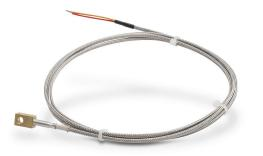
ProSense temperature sensor, Type J thermocouple, bolt-on ring, ungrounded junction, brass sheath, #6 - #10 (4-5mm) screw or bolt size process connection, 6ft 20 AWG wire leads.
