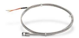
ProSense temperature sensor, Type J thermocouple, bolt-on ring, grounded, stainless steel sheath, #6 to #10 (4mm to 5mm) screw or bolt size process connection, 6ft 20 AWG wire leads.
