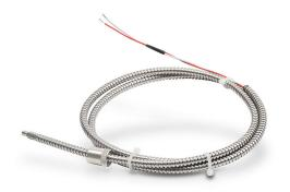
ProSense temperature sensor, Type J thermocouple, armor adjustable immersion probe, ungrounded, 1/4in insertion length, 3/16in probe diameter, stainless steel sheath, bayonet cap process connection, 10ft 20 AWG wire leads.
