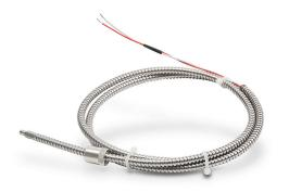
ProSense temperature sensor, Type J thermocouple, armor adjustable immersion probe, grounded, 1/4in insertion length, 3/16in probe diameter, stainless steel sheath, bayonet cap process connection, 10ft 20 AWG wire leads.
