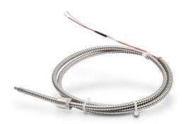
ProSense temperature sensor, Type J thermocouple, armor adjustable immersion probe, grounded, 1/4in insertion length, 3/16in probe diameter, stainless steel sheath, bayonet cap process connection, 6ft 20 AWG wire leads.
