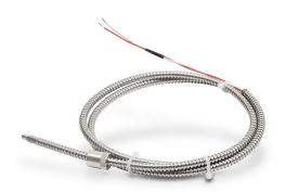
ProSense temperature sensor, Type J thermocouple, armor adjustable immersion probe, grounded, 1/4in insertion length, 3/16in probe diameter, stainless steel sheath, bayonet cap process connection, 4ft 20 AWG wire leads.
