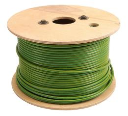
Atlas Wire THHN building wire, single conductor, 8 AWG, 19-stranded, bare copper, PVC conductor insulation material, green with yellow stripe, nylon jacket, clear, 600V, 500ft reel.
