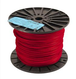
Atlas Wire THHN building wire, single conductor, 14 AWG, 19-stranded, bare copper, PVC conductor insulation material, red, nylon jacket, clear, 600V, 500ft spool.
