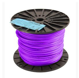
Atlas Wire THHN building wire, single conductor, 14 AWG, 19-stranded, bare copper, PVC conductor insulation material, purple, nylon jacket, clear, 600V, 500ft spool.
