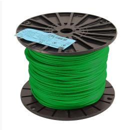
Atlas Wire THHN building wire, single conductor, 14 AWG, 19-stranded, bare copper, PVC conductor insulation material, green, nylon jacket, clear, 600V, 500ft spool.
