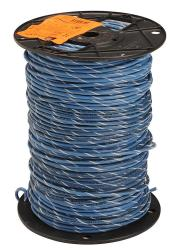
Atlas Wire THHN building wire, single conductor, 14 AWG, 19-stranded, bare copper, PVC conductor insulation material, blue with white stripe, nylon jacket, clear, 600V, 500ft spool.
