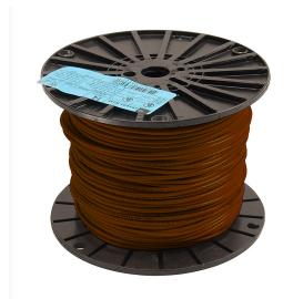
Atlas Wire THHN building wire, single conductor, 14 AWG, 19-stranded, bare copper, PVC conductor insulation material, brown, nylon jacket, clear, 600V, 500ft spool.
