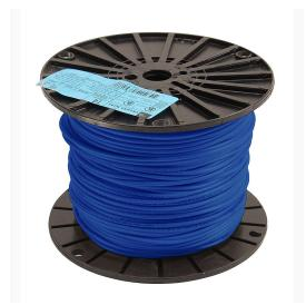
Atlas Wire THHN building wire, single conductor, 14 AWG, 19-stranded, bare copper, PVC conductor insulation material, blue, nylon jacket, clear, 600V, 500ft spool.
