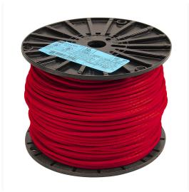
Atlas Wire THHN building wire, single conductor, 12 AWG, 19-stranded, bare copper, PVC conductor insulation material, red, nylon jacket, clear, 600V, 500ft spool.
