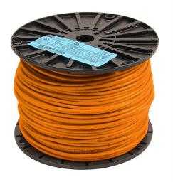
Atlas Wire THHN building wire, single conductor, 12 AWG, 19-stranded, bare copper, PVC conductor insulation material, orange, nylon jacket, clear, 600V, 500ft spool.
