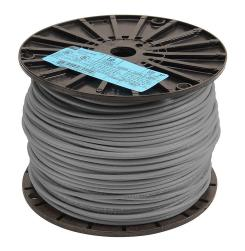
Atlas Wire THHN building wire, single conductor, 12 AWG, 19-stranded, bare copper, PVC conductor insulation material, gray, nylon jacket, clear, 600V, 500ft spool.
