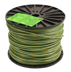
Atlas Wire THHN building wire, single conductor, 12 AWG, 19-stranded, bare copper, PVC conductor insulation material, green with yellow stripe, nylon jacket, clear, 600V, 500ft spool.
