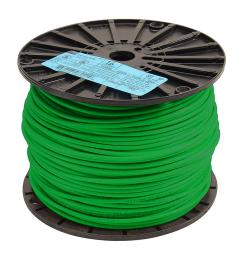
Atlas Wire THHN building wire, single conductor, 12 AWG, 19-stranded, bare copper, PVC conductor insulation material, green, nylon jacket, clear, 600V, 500ft spool.
