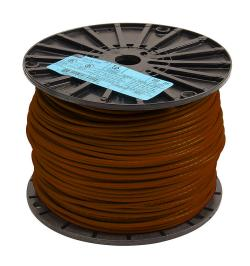
Atlas Wire THHN building wire, single conductor, 12 AWG, 19-stranded, bare copper, PVC conductor insulation material, brown, nylon jacket, clear, 600V, 500ft spool.
