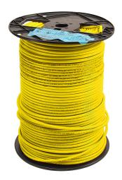
Atlas Wire THHN building wire, single conductor, 10 AWG, 19-stranded, bare copper, PVC conductor insulation material, yellow, nylon jacket, clear, 600V, 500ft spool.
