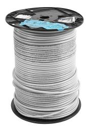
Atlas Wire THHN building wire, single conductor, 10 AWG, 19-stranded, bare copper, PVC conductor insulation material, white, nylon jacket, clear, 600V, 500ft spool.
