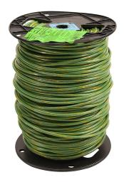
Atlas Wire THHN building wire, single conductor, 10 AWG, 19-stranded, bare copper, PVC conductor insulation material, green with yellow stripe, nylon jacket, clear, 600V, 500ft spool.
