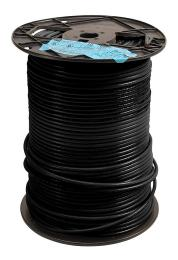
Atlas Wire THHN building wire, single conductor, 10 AWG, 19-stranded, bare copper, PVC conductor insulation material, black, nylon jacket, clear, 600V, 500ft spool.
