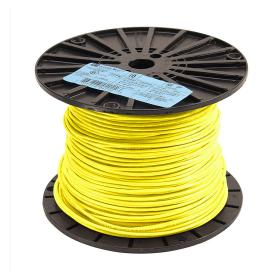
Atlas Wire TFFN building wire, single conductor, 18 AWG, 16-stranded, bare copper, PVC conductor insulation material, yellow, nylon jacket, clear, 600V, 500ft spool.
