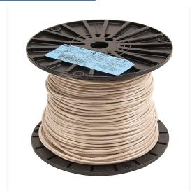
Atlas Wire TFFN building wire, single conductor, 18 AWG, 16-stranded, bare copper, PVC conductor insulation material, white, nylon jacket, clear, 600V, 500ft spool.
