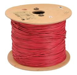
Atlas Wire TFFN building wire, single conductor, 18 AWG, 16-stranded, bare copper, PVC conductor insulation material, red, nylon jacket, clear, 600V, 2500ft reel.
