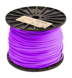
Atlas Wire TFFN building wire, single conductor, 18 AWG, 16-stranded, bare copper, PVC conductor insulation material, purple, nylon jacket, clear, 600V, 500ft spool.
