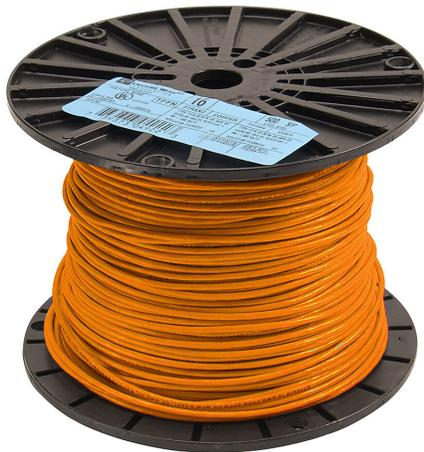
Atlas Wire TFFN building wire, single conductor, 18 AWG, 16-stranded, bare copper, PVC conductor insulation material, orange, nylon jacket, clear, 600V, 500ft spool.
