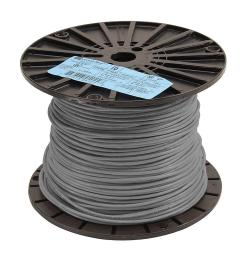
Atlas Wire TFFN building wire, single conductor, 18 AWG, 16-stranded, bare copper, PVC conductor insulation material, gray, nylon jacket, clear, 600V, 500ft spool.
