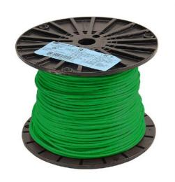
Atlas Wire TFFN building wire, single conductor, 18 AWG, 16-stranded, bare copper, PVC conductor insulation material, green, nylon jacket, clear, 600V, 500ft spool.
