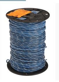
Atlas Wire TFFN building wire, single conductor, 18 AWG, 16-stranded, bare copper, PVC conductor insulation material, blue with white stripe, nylon jacket, clear, 600V, 500ft spool.
