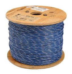
Atlas Wire TFFN building wire, single conductor, 18 AWG, 16-stranded, bare copper, PVC conductor insulation material, blue with white stripe, nylon jacket, clear, 600V, 2500ft reel.
