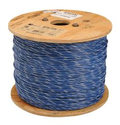
Atlas Wire TFFN building wire, single conductor, 18 AWG, 16-stranded, bare copper, PVC conductor insulation material, blue with white stripe, nylon jacket, clear, 600V, 2500ft reel.
