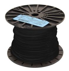
Atlas Wire TFFN building wire, single conductor, 18 AWG, 16-stranded, bare copper, PVC conductor insulation material, black, nylon jacket, clear, 600V, 500ft spool.
