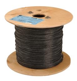
Atlas Wire TFFN building wire, single conductor, 18 AWG, 16-stranded, bare copper, PVC conductor insulation material, black, nylon jacket, clear, 600V, 2500ft reel.
