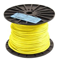
Atlas Wire TFFN building wire, single conductor, 16 AWG, 26-stranded, bare copper, PVC conductor insulation material, yellow, nylon jacket, clear, 600V, 500ft spool.
