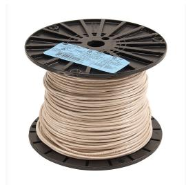
Atlas Wire TFFN building wire, single conductor, 16 AWG, 26-stranded, bare copper, PVC conductor insulation material, white, nylon jacket, clear, 600V, 500ft spool.
