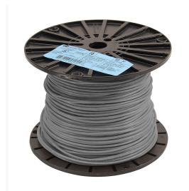
Atlas Wire TFFN building wire, single conductor, 16 AWG, 26-stranded, bare copper, PVC conductor insulation material, gray, nylon jacket, clear, 600V, 500ft spool.
