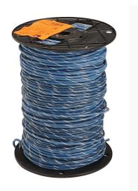
Atlas Wire TFFN building wire, single conductor, 16 AWG, 26-stranded, bare copper, PVC conductor insulation material, blue with white stripe, nylon jacket, clear, 600V, 500ft spool.
