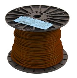
Atlas Wire TFFN building wire, single conductor, 16 AWG, 26-stranded, bare copper, PVC conductor insulation material, brown, nylon jacket, clear, 600V, 500ft spool.
