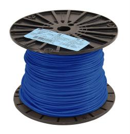
Atlas Wire TFFN building wire, single conductor, 16 AWG, 26-stranded, bare copper, PVC conductor insulation material, blue, nylon jacket, clear, 600V, 500ft spool.
