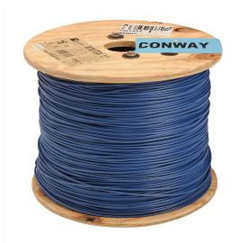
Atlas Wire TFFN building wire, single conductor, 16 AWG, 26-stranded, bare copper, PVC conductor insulation material, blue, nylon jacket, clear, 600V, 2500ft reel.
