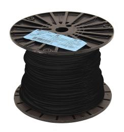
Atlas Wire TFFN building wire, single conductor, 16 AWG, 26-stranded, bare copper, PVC conductor insulation material, black, nylon jacket, clear, 600V, 500ft spool.
